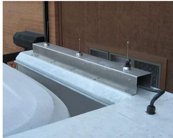
The antenna mounting platform projects vertically lower than the escape or vent hatch seen towards the front of the vehicle; height was calculated to make certain the new mounting structure did not become the tallest element of the vehicle system. Where does this all lead? A view of the Operator's position appears below:
